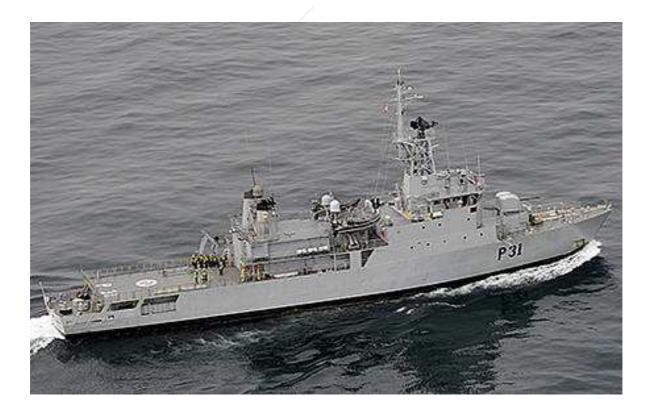
Below is LE Samuel Beckett. This is one of the newer, more powerful and faster additions to the NS fleet. The Agusta 139 is used for vertical supply of this ship also. The area for depositing the underslung load is the stern (aft) deck. As can be seen, this is quite close to the single exhaust stack. During these operations, the helicopter is hovering approximately level with the top of the exhaust stack. At full power these engines have an output of 55% of the proposed plant at Ringaskiddy.
